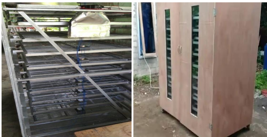
Figure 1. The inner and outer framework of an energy-saving automatic hatching machine (Source: Personal documentation)
